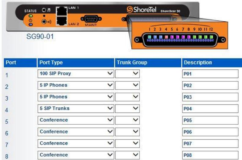
**Figure 15 – ShoreGear Switch Settings**
