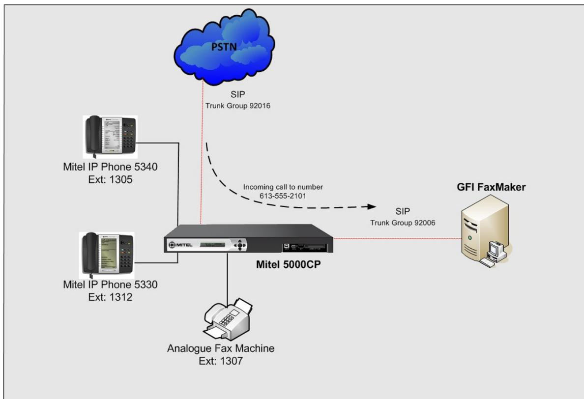
**Figure 10 – The configuration with two SIP trunks**
