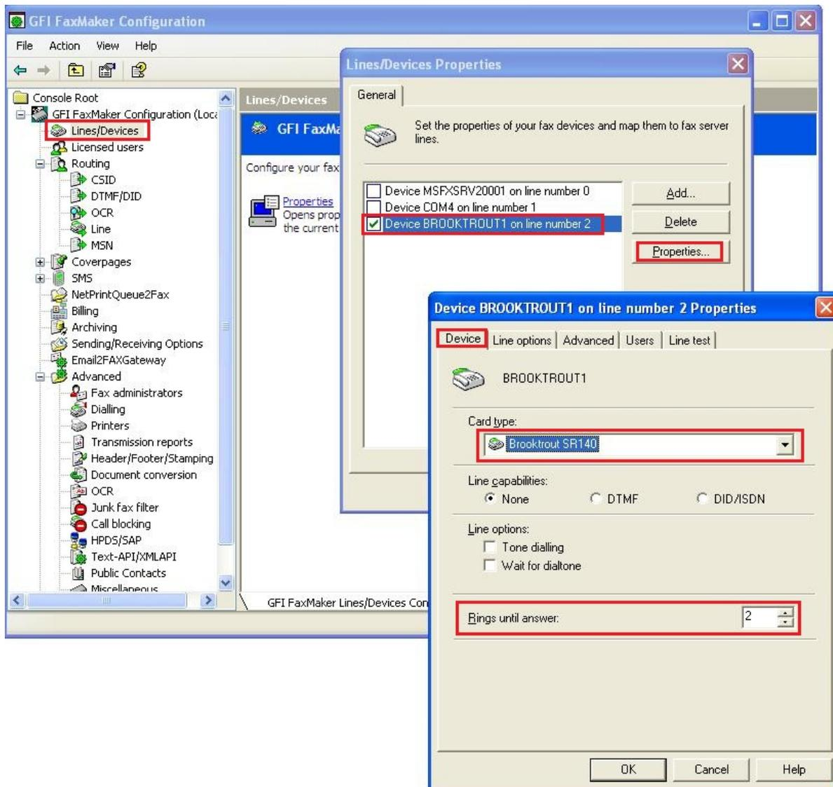
**Figure 15 – Configuration settings for Brooktrout SR140' line**
