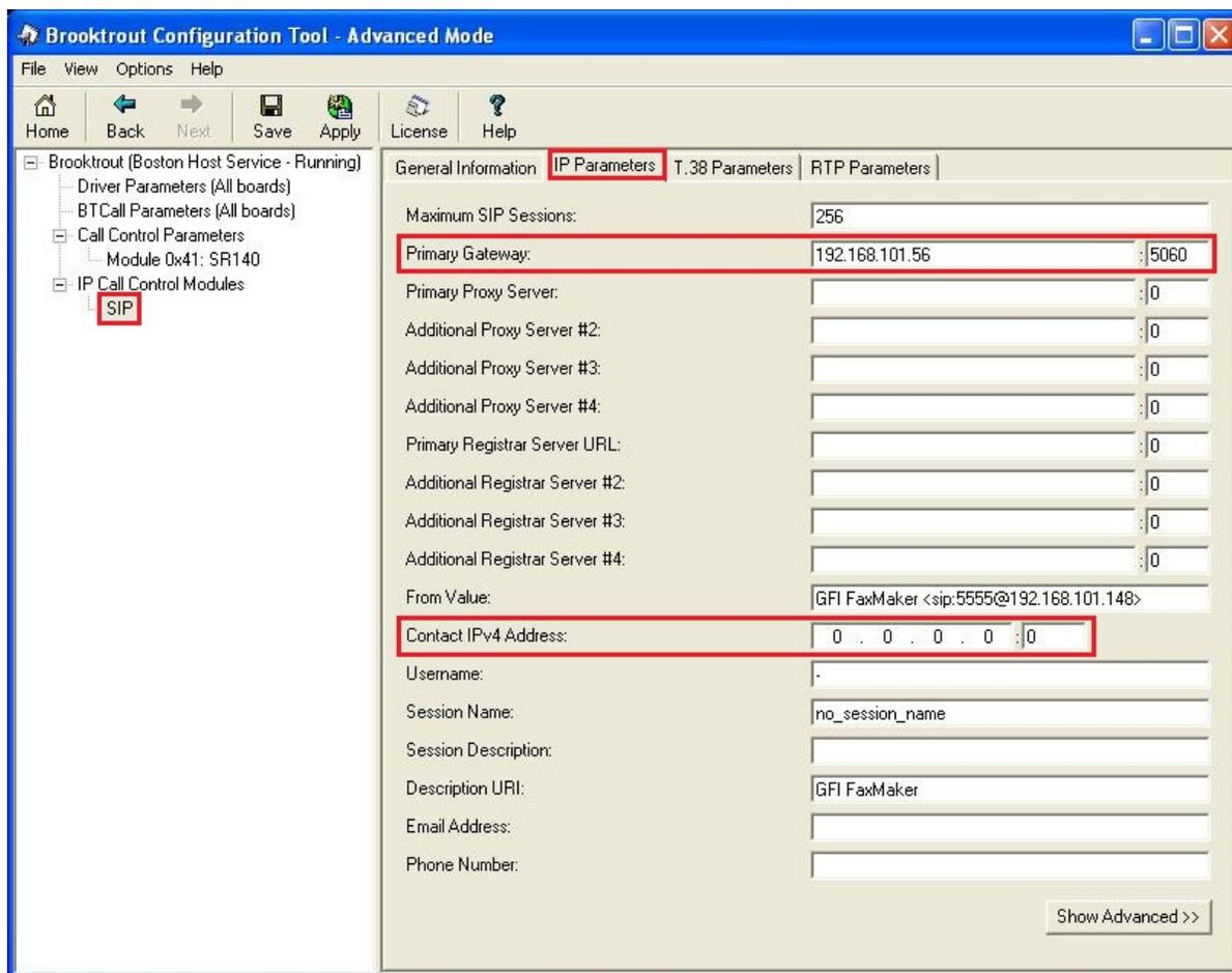
Figure 18 – IP Parameters’ settings for Brooktrout SR140
