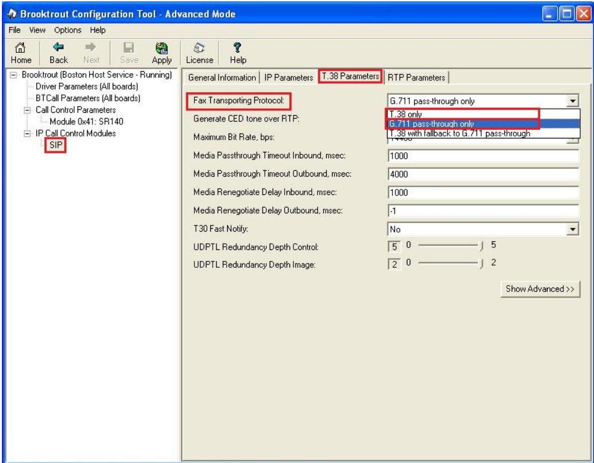
Figure 19 – T.38 Parameters' settings for Brooktrout SR140
